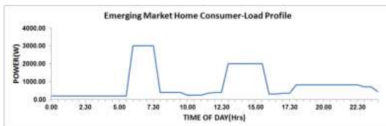
Figure 1. Typical emerging market home load curve.
